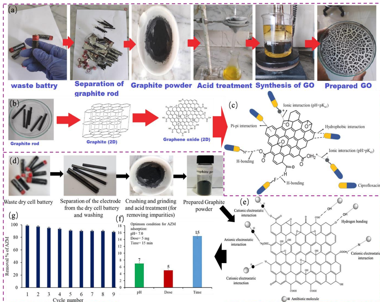
Figure 4: (a) Preparation process of GO from spent Zn–C batteries. (b) Structure of the graphite rod. (c) Proposed mechanism for CIP removal using GO [62]. (d) Synthetic process of GO derived from spent dry batteries. (e) Morphological structure of the graphite rod and possible removal mechanism for AZM. (f) Determination of optimal adsorption conditions for AZM. (g) Reusability performance of GO for AZM removal over nine cycles [120].
